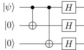
Here,  $|0\rangle$  means that the two auxiliary qubits are initialized in  $|0\rangle$ . The decoding scheme is the inverse of the encoding scheme. Finally, the actual error correction is performed by a single Toffoli gate with the two auxiliary qubits as the control qubits and the original qubit as the target.
